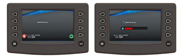
**9.** Allow the display to automatically reboot when you see the Check Mark Screen momentarily.
