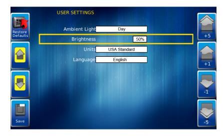
**NOTE**: Brightness level will change with ambient light setting. Two brightness levels are saved; one for day and one for night.
