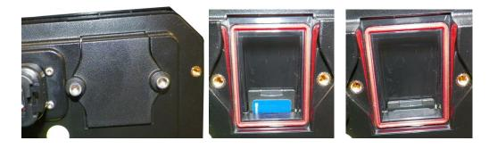
6. With the USB drive or the SD card installed, press and hold the enter key (bottom right) on the display for a few seconds as you Power-on the display. The system will boot up in configuration mode.
